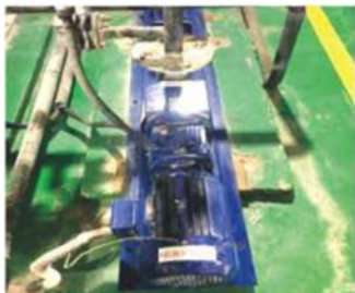
Screw pump is used in lime milk industry
