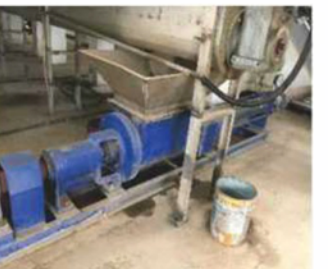
Dry mud pump is used after dehydration
