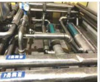
Food-grade screw pump is used to transport jam
